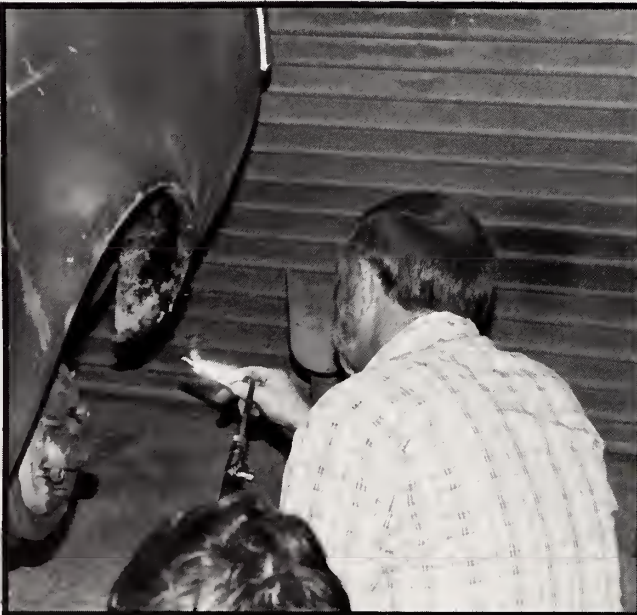
Instructor for the Auto Body Repair program, Gerald Wood, demonstrates a perplexive procedure for body leading.
