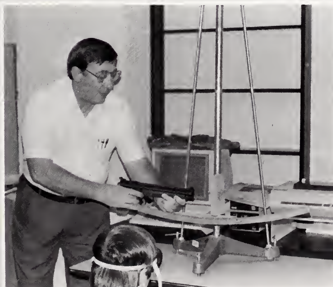
Mr. Robert Walker, physics instructor, is demonstrating the pendulum apparatus to the physics students. The experiment for the day was using the inelastic impact pendulum to study the velocity of a projectile.
