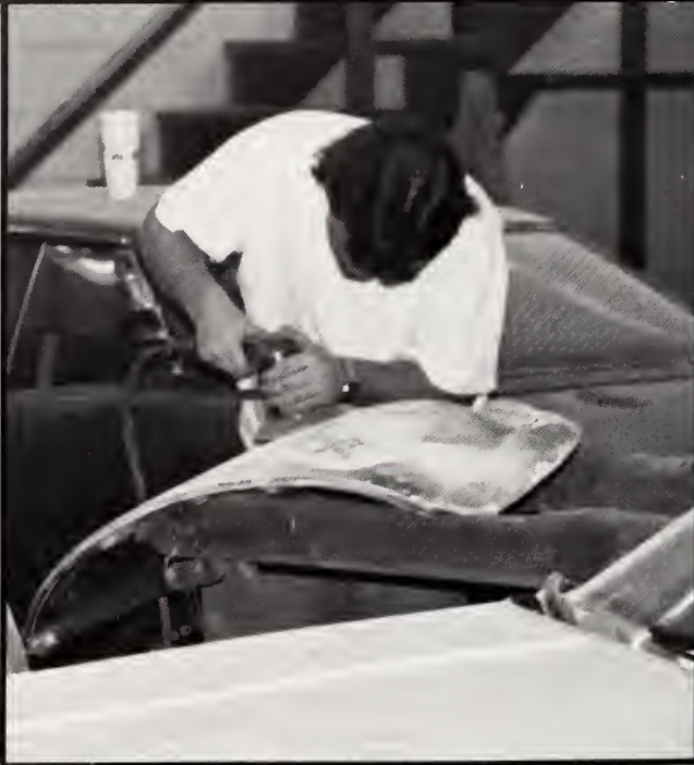
Operating a "D.A." sander, Auto Body Repair student, Bobby Shew, applies his skill while sanding down the fender of a volkswagon.
