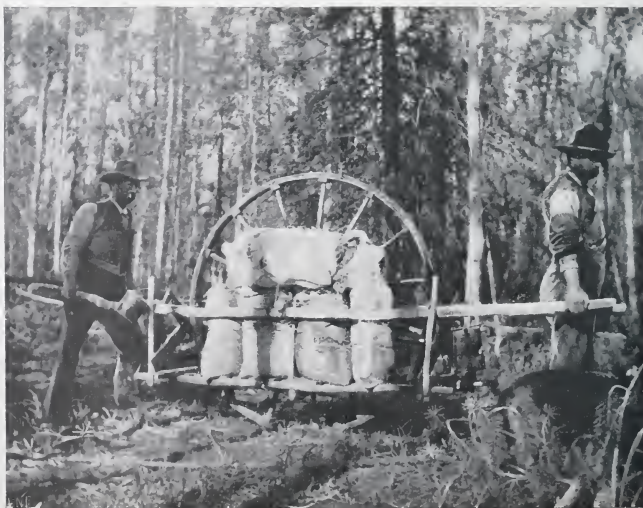
A UNIQUE MODE OF LOCOMOTION THROUGH THE FORESTS AND SWAMPS. THIS IS A TYPICAL "GO-DEVIL" MADE BY THE MINERS. [Photo.]
