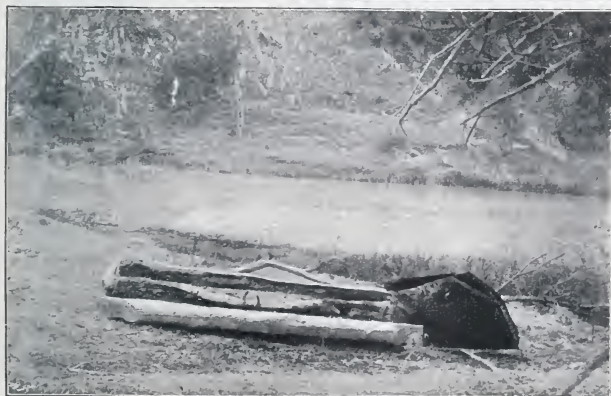
BOAT MADE OUT OF AN AUSTRALIAN MINER'S PUDDLING-TROUGH. THE ROWLOCKS ARE INVERTED HORSE-SHOES. From a Photo.
