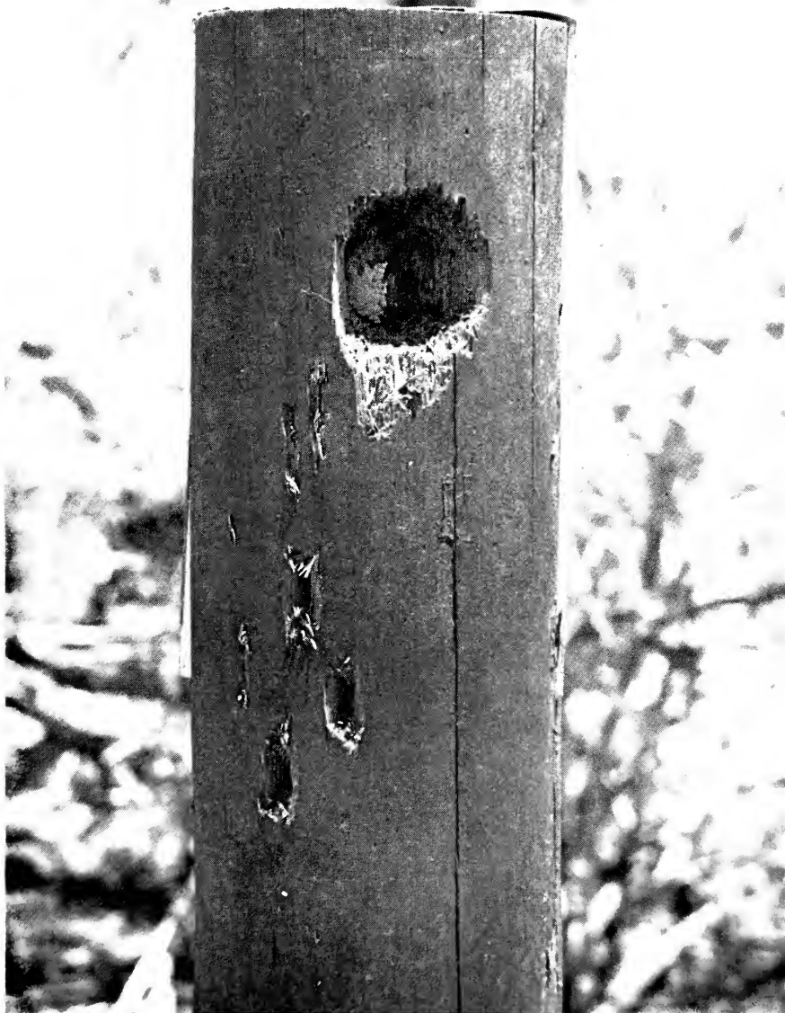
FIG. 3. A flat metal plate has been inserted into a groove cut into the top of this creosoted pine fence post. A woodpecker has drilled a hole to the plate. Small holes are scattered about near the large hole.
