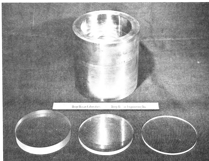
Figure 4. Flat acrylic windows and 4.00-inch ( D_i ) flange used to determine the relationship between the window's critical pressure and t/D_i ratio.
