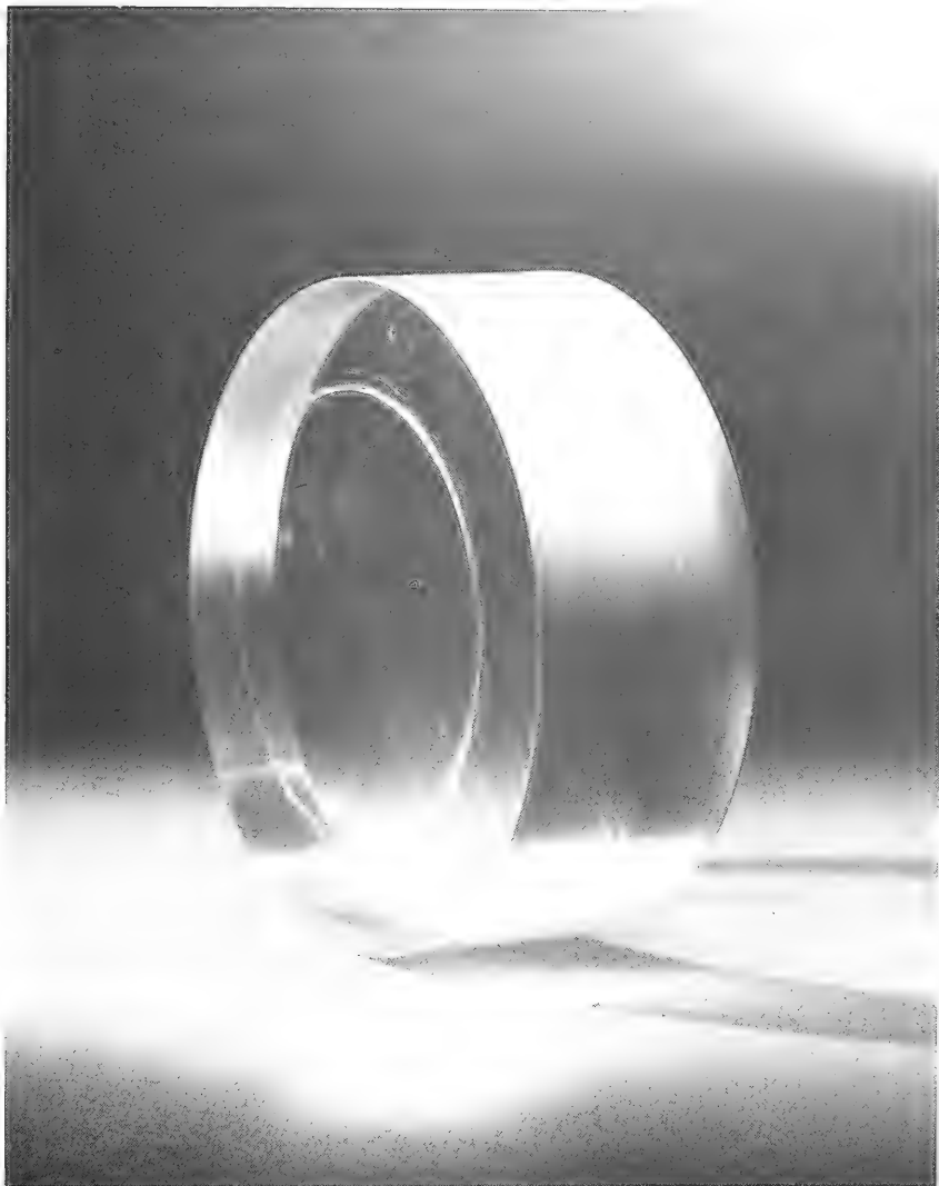
Figure B-26. Permanent extrusion of low-pressure face of a flat acrylic window having a 0.490 t/D_i ratio; window pressurized to 67% of ultimate critical pressure.
