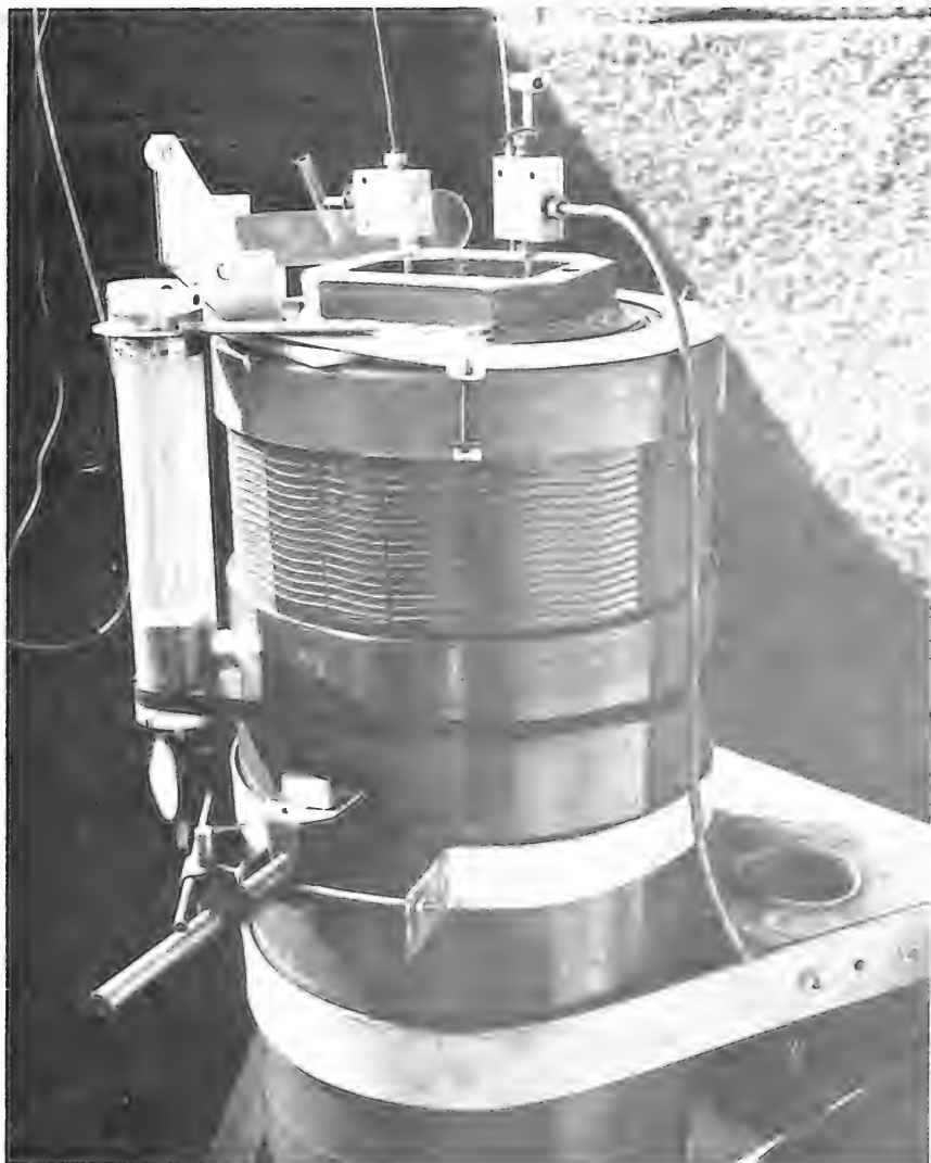
Figure 7. Deflection-measuring apparatus in place on pressure vessel.
