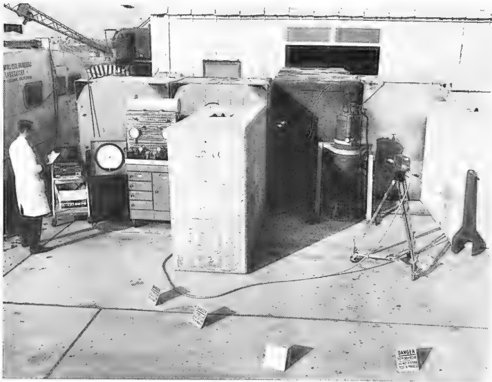
Figure 9. Pressure gages, pumps, and closed-circuit television monitor used behind barricade during testing.
