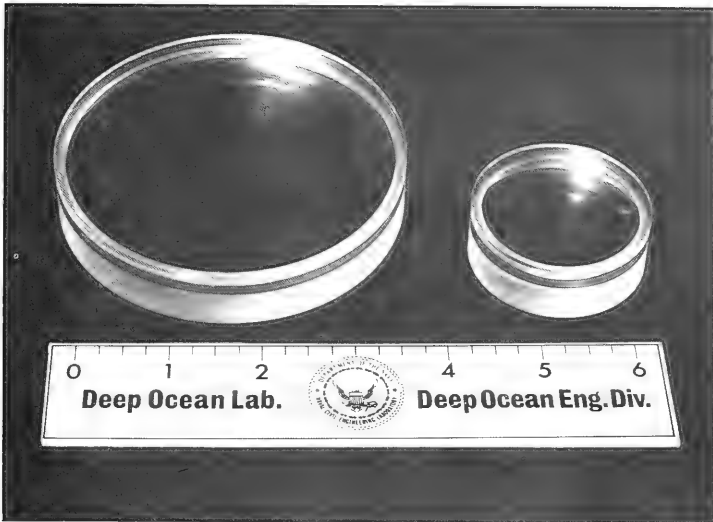
Figure A-4. Flat acrylic windows used with O-ring sealing technique in the investigation of window mountings.
