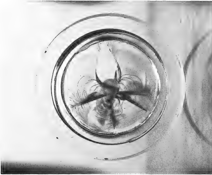
Figure B-8. Coalescing conchoidal fractures just prior to failure in a 0.735-inch-thick window with a t/D_i ratio of 0.490; maximum pressurization 18,600 psi.
