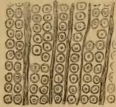
FIG. 166.—Longitudinal section of pine-wood, parallel to a medullary ray; showing the rows of ducts.
