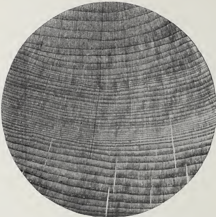
Fig. 15. Cross-section of Non-porous Wood, White Pine, Full Size (top toward pith).
