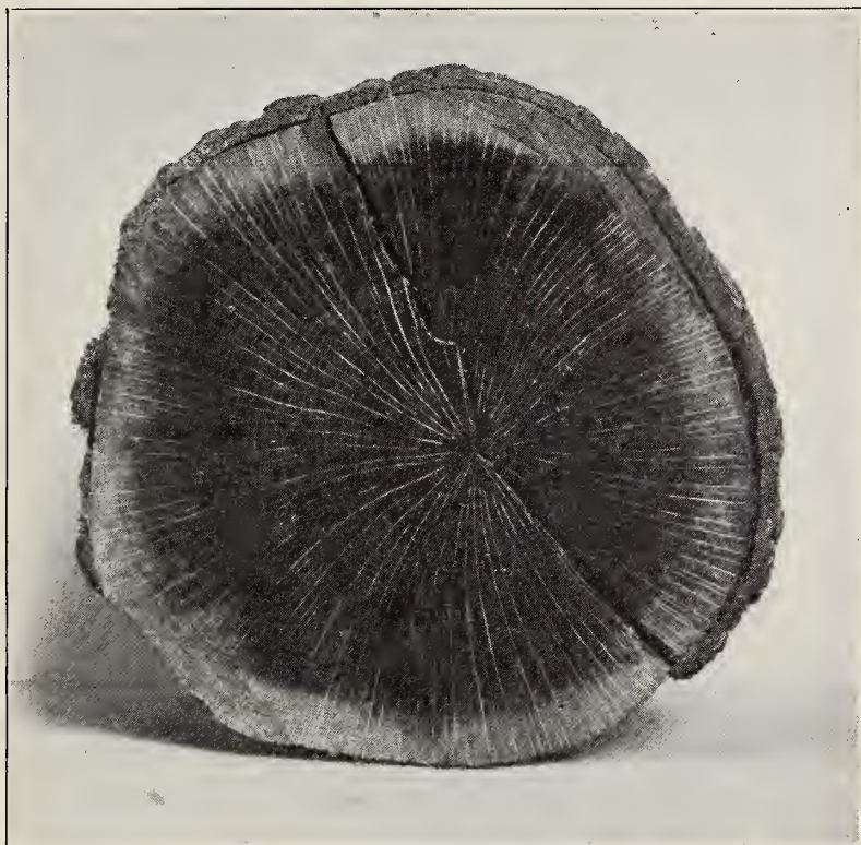
Fig. 14 Cross-section of White Oak. The Radiating White Lines are the Pith Rays.
