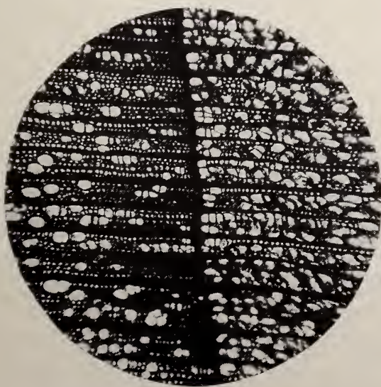
Cross-section, magnified 37\frac{1}{2} diameters.
