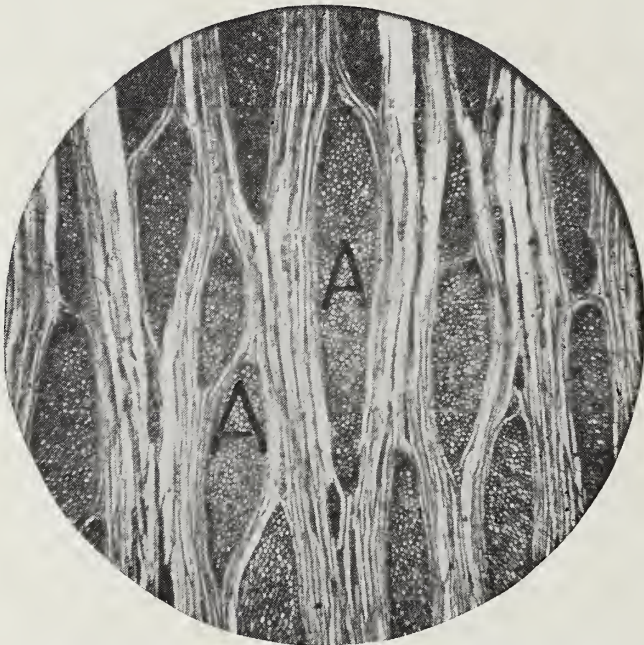
Fig. 13. Tangential Section of Sycamore, Magnified 37 Diameters. Note the large size of the pith rays, A, A (end view).
