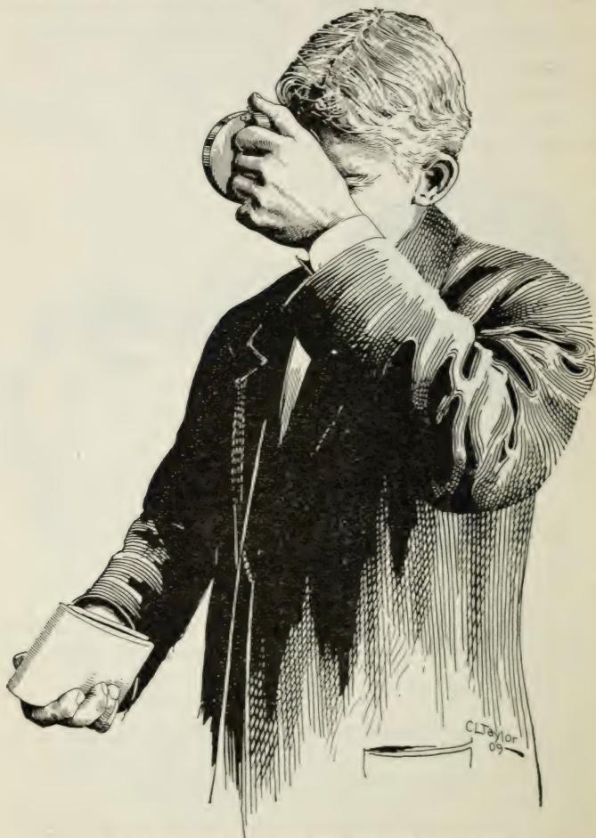
FIG. 10.—Method of sighting with standard hypsometer.
