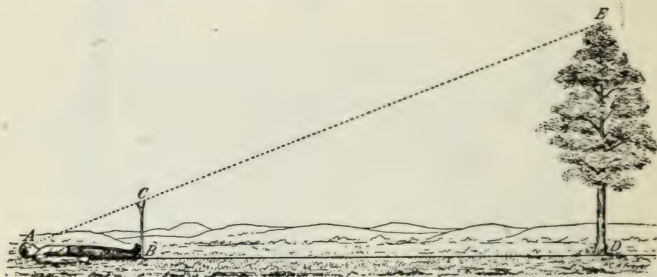
FIG. 7.—Measuring the height of a tree by use of known height to eye of the observer.
