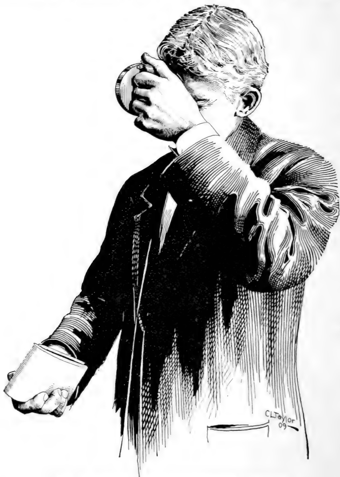
FIG. 10.—Method of sighting with standard hypsometer.
