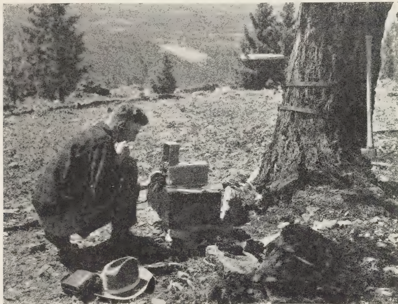
FIGURE 16.—Patrolman using Forest Service field radio set on lookout point. Portable map board and alidade are strapped to tree. Lolo National Forest, Mont.
