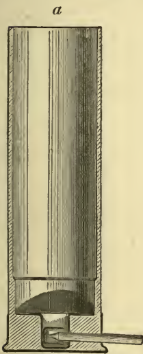
SECTION OF PIN CARTRIDGE CASE.
