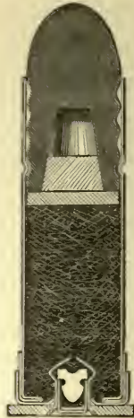
SECTION OF "BOXER" CARTRIDGE, ·577 BORE.
