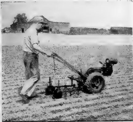
Field Scene 2½ H.P. Tractor with Cultivator
