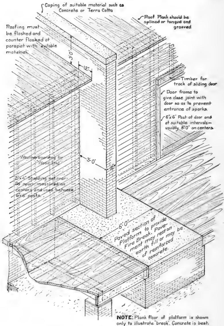
FIG. 29.—Division fire wall arranged as an economical fire stop.
