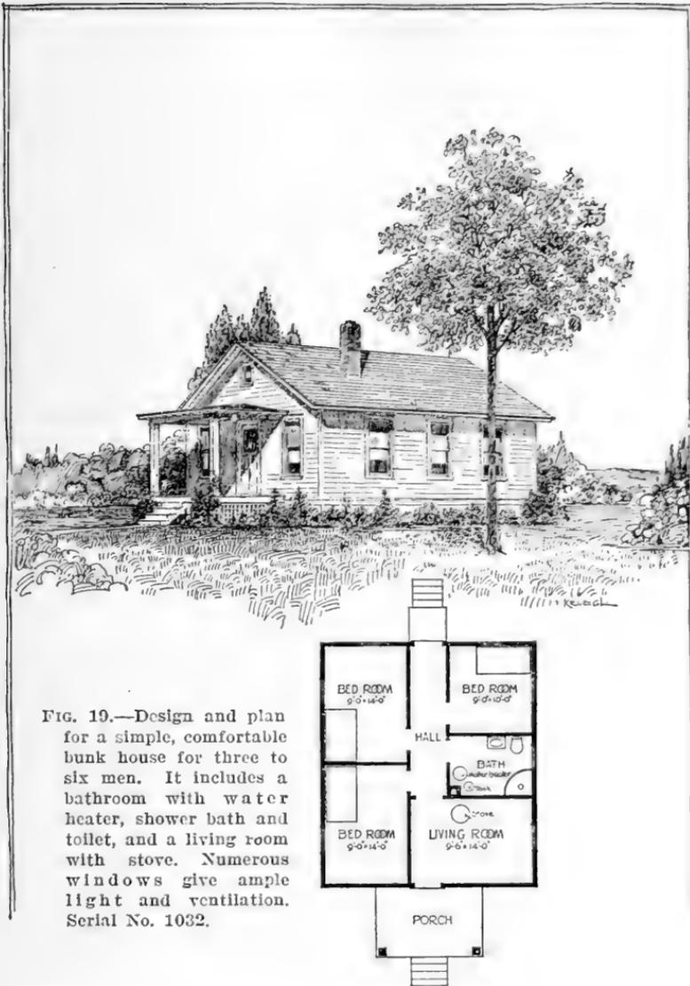
FIG. 19.—Design and plan for a simple, comfortable bunk house for three to six men. It includes a bathroom with water heater, shower bath and toilet, and a living room with stove. Numerous windows give ample light and ventilation. Serial No. 1032.
