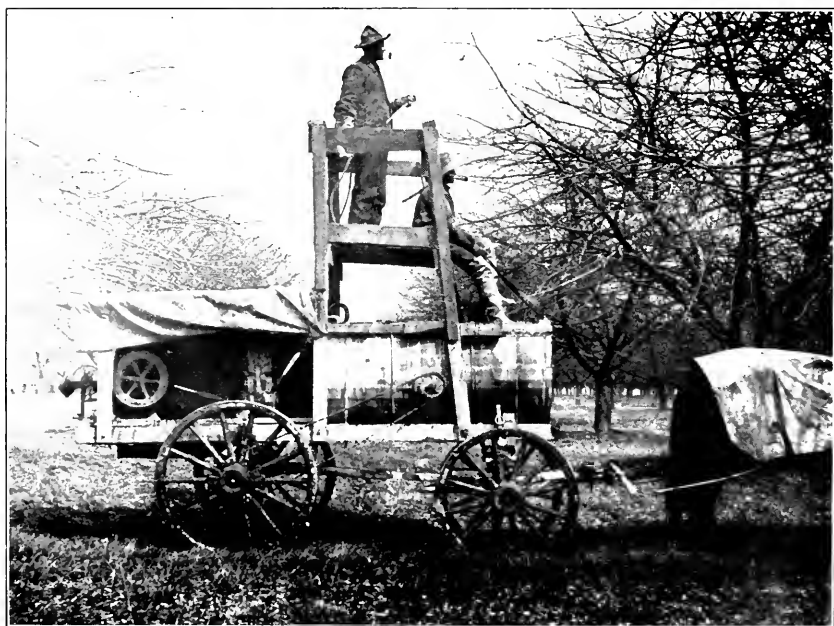
FIG. 2.—A GASOLINE POWER OUTFIT USED IN WESTERN NEW YORK. (ORIGINAL.) OUTFITS USED FOR SPRAYING LIME-SULPHUR WASH.
