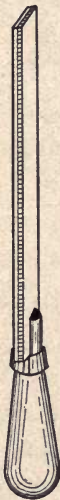
Fig. 7. A bar which is made of two different metals, bends when it is heated, because one of the metals expands more rapidly than the other.
