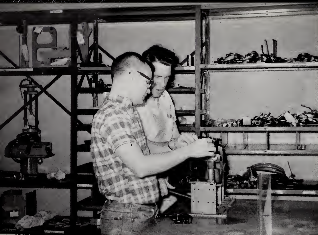
C. C. Price and John Marshall are checking an injector plunger for seating properly in the injector cup.
